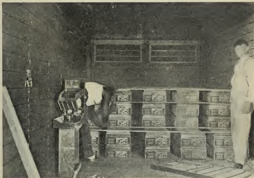
Fig. 22.—Interior of a standard refrigerator car showing the manner of loading and "stripping."
